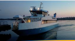
The 28 m ferry is built with steel hull and aluminum superstructure. The hull and its propulsion is made for operation in ice conditions. A strong bow thruster and two main engines offers good maneuverability in congested harbors. The passenger cabin has an open layout with 110 seats and 50 seats on weather deck. Aft of the passenger cabin there is a large cargo deck area with a crane for loading and unloading. Cargo is handled via the bow ramp.
