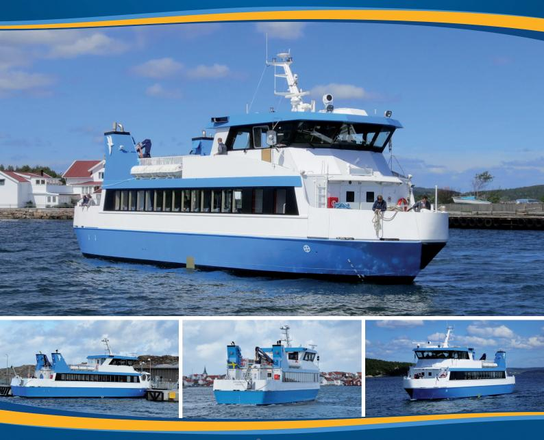
The 24 m ferry is built with a steel hull and an aluminum superstructure. The propulsion is two 13 litre Scania engines in combination with fixed pitch propellers and a bow thruster. The passenger cabin has an open layout with 99 seats and 49 seats on the weather deck. Aft of the passenger cabin there is a large cargo deck area with a crane for loading and unloading. Wheeled cargo could be handled via the bow ramp.
