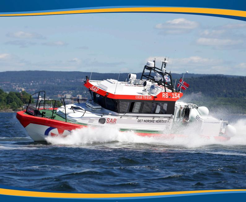
High speed rescue craft. Low wake-wash, energy efficient High towing capacity. Excellent maneuvering with waterjet Glass fiber composite hull, full sandwich.
