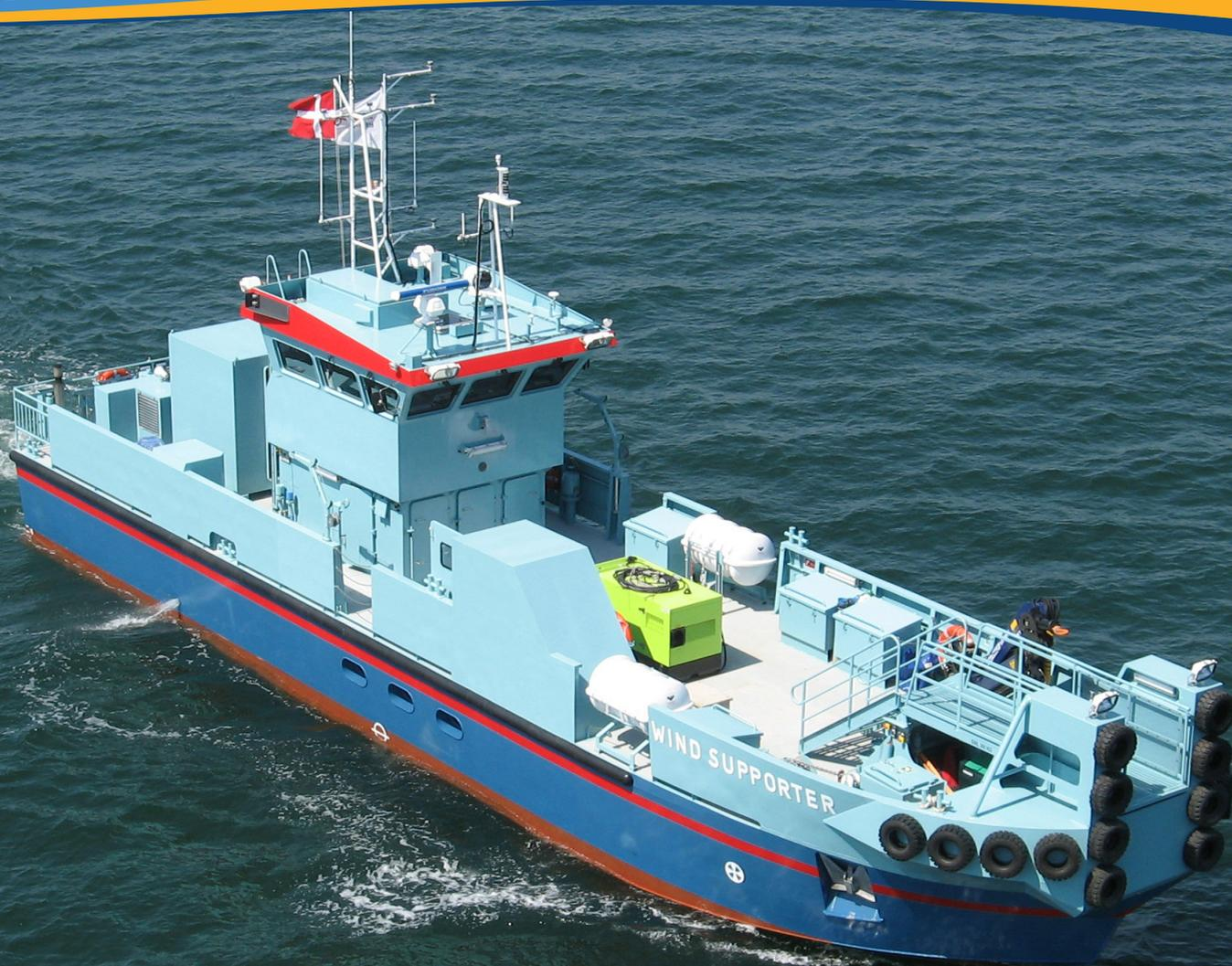
Wind Supporter is a Service vessel made for bow mooring on offshore wind mills and fitted with a 2 mT crane. The vessel is designed and built according to DNV rules with an operating range of 20 M from the shore line and to the DMA rules allowing for 24 passengers.
