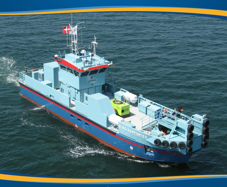
Wind Supporter is a Service vessel made for bow mooring on offshore wind mills and fitted with a 2 mT crane. The vessel is designed and built according to DNV rules with an operating range of 20 M from the shore line and to the DMA rules allowing for 24 passengers.
