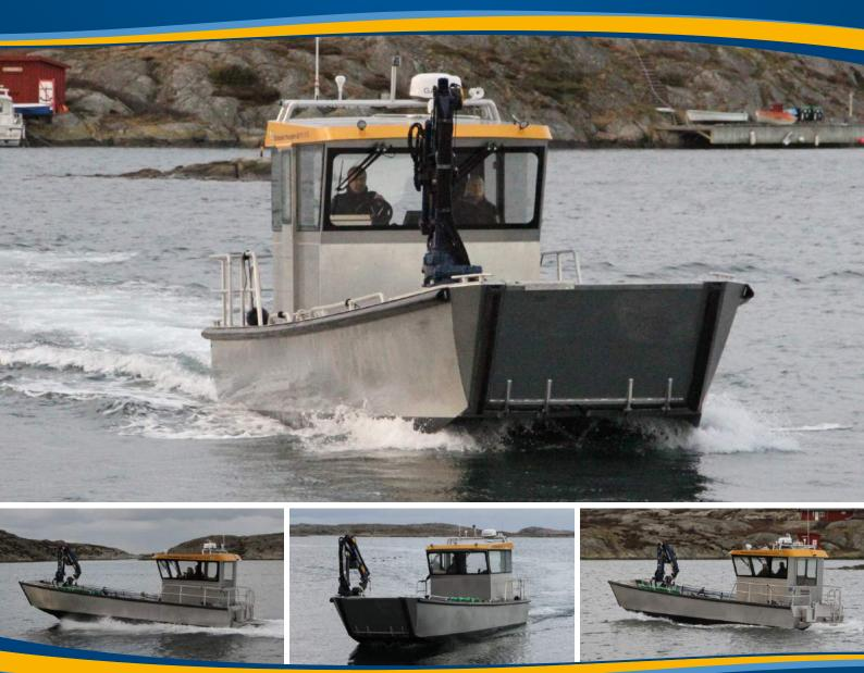
A robust waterjet driven work boat designed for commercial use. The boat is equipped with a crane, has a reinforced keel and bow ramp allowing for loading and unloading from the beach. Typical usage is for towing, taxi, support, cargo, fish farming, diving, rescue operation and oil recovery.
